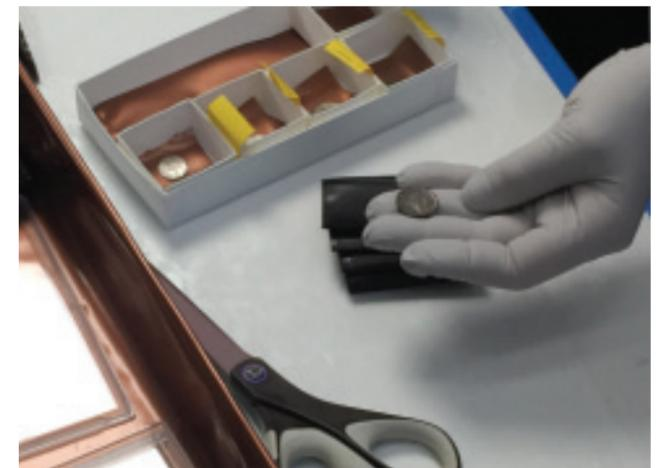
The artifacts are prepared to the science of our day: each item is enveloped in a corrosion intercepting material and separated by a pure cellulose sheet. No oxygen is in the box: only slightly humidified argon, an inert gas.
