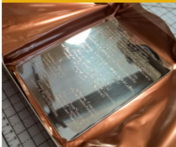
box would remain separate from the new box, and to that end it had been encapsulated in a protective envelope of Reactive Intercept Barrier System (RIBS) foil (a moisture and oxygen barrier film) and placed into the cornerstone before the start of the formal activities.
